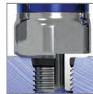
**1. SAE Straight Thread O-Ring (ORB).** This parallel thread termination follows SAE J1926 – an industry specification for fluid ports utilizing ASME B1.1 thread profiles. It features elastomeric sealing and is commonly used in North America.
