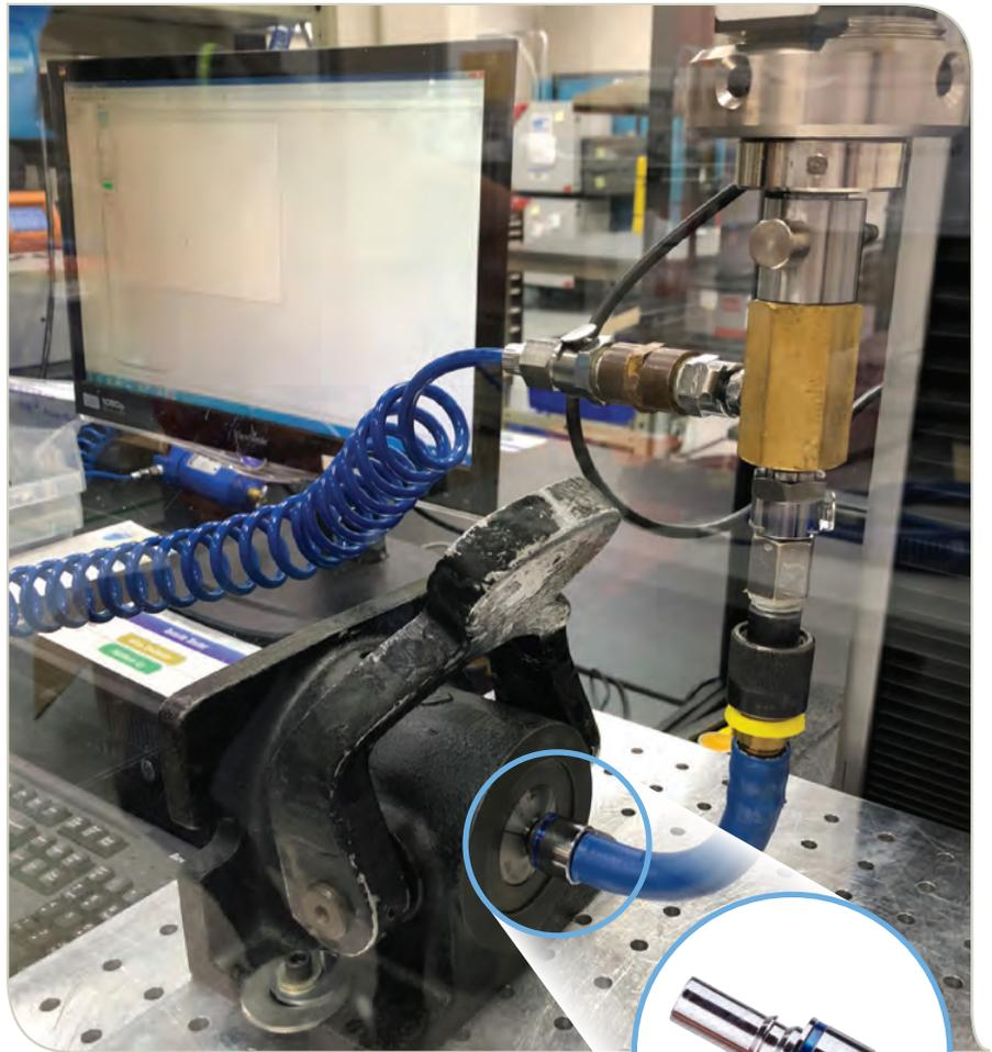
tubing like EPDM. They also avoid leakage under side load (in excess of ~200lbf). Hose assembly with locking barbs often requires more force than traditional triple barbs. Light application of heat or lubricant may ease installation. Typical removal of hydraulic-type hose from this style of termination requires cutting along the length of the barb with a thin blade, taking care not to scratch or damage the barb, especially on any of the sealing surfaces.
