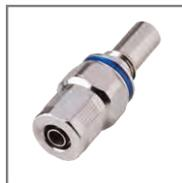
**3. Compression.** Common compression style terminations include a ring or ferrule to mate with rigid tubing, and a nut to thread capture the ferrule against the termination seat.
