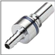
**1. Triple barb.** Fluid coupling terminations with multiple, shallow barbs are commonly used with lighter weight tubing. The triple barb design
